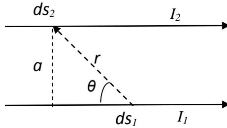
Fig.4. The charge  $dq_1$  is located on the segment  $ds_1$ , while the charge  $dq_2$  is on the segment  $ds_2$ .
