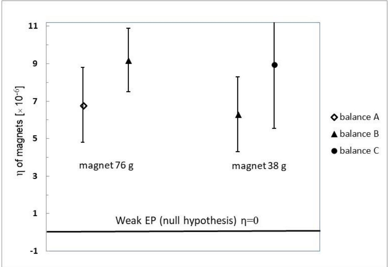
FIG. 2: The graph shows relative differences  $\eta = \Delta W / W$  of the vertical and horizontal weights of two neodymium magnets. The error bars refer to the statistical standard deviations. All horizontal orientations of the magnets are East-West.
