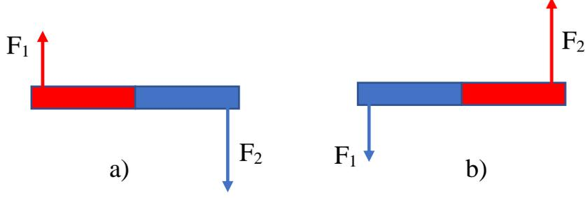
FIG. 1: Influence of an inhomogeneous terrestrial magnetic field on a bar magnet in two opposite orientations: a) the magnetization axis is directed to the East; b) the magnetization axis is directed to the West.
